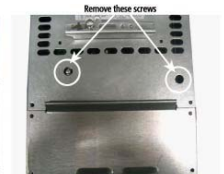
Figure 5.h - Changing of EMC protection class, MF6
