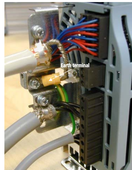
Figure 6.i. Cable installation for MF3
